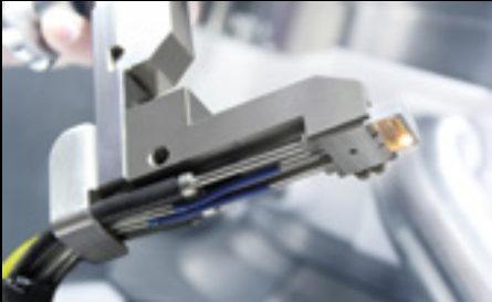
NIR sensors in the tablet press analyze the concentration of active ingredient of the products.
