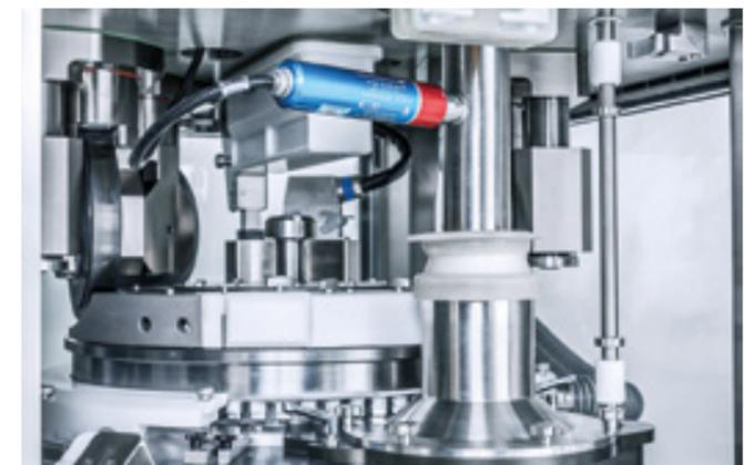
Raman measuring in tablet press
