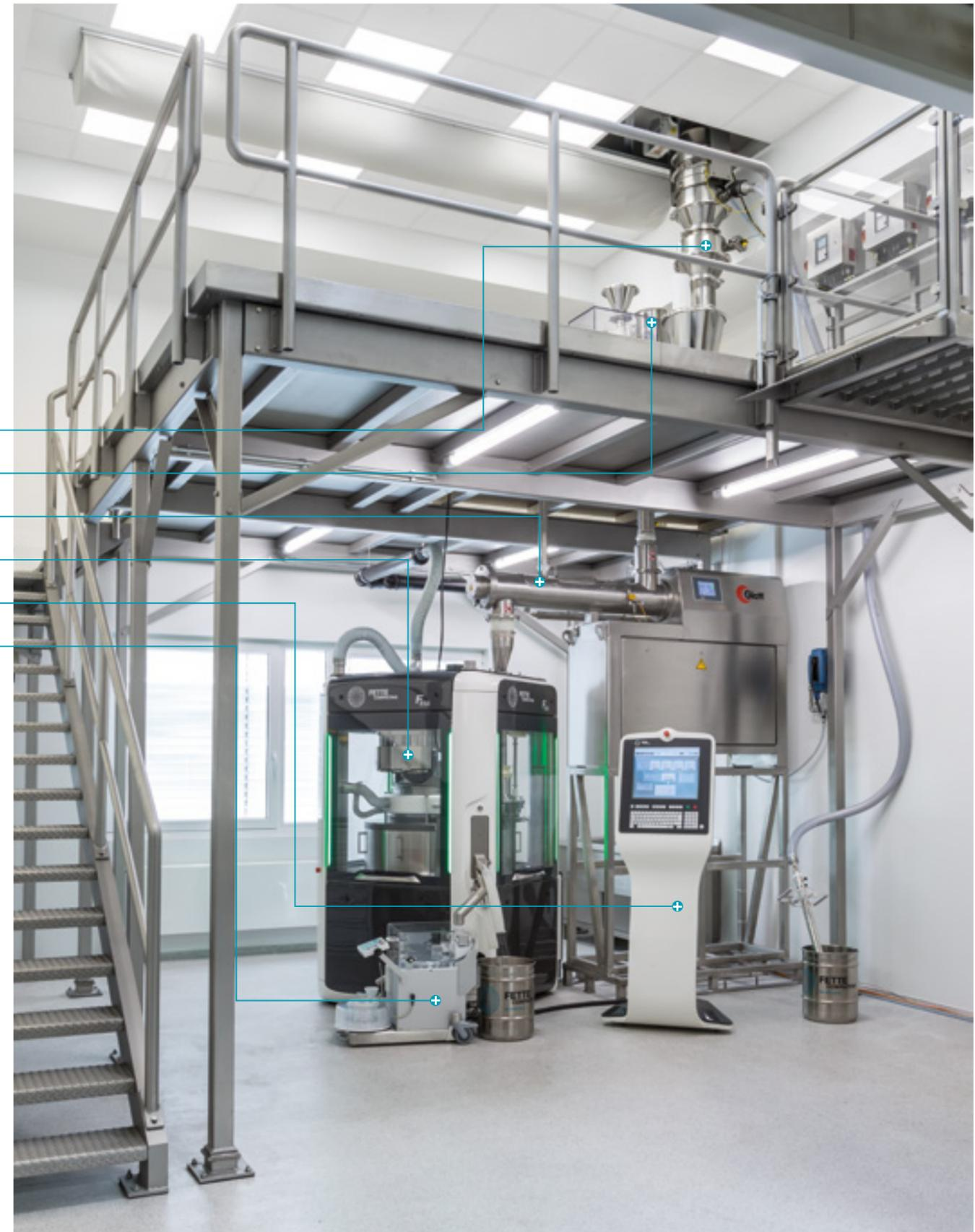
Direct compression line supplied by Fette Compacting: FE55 tablet press with dosing unit and mixing system
