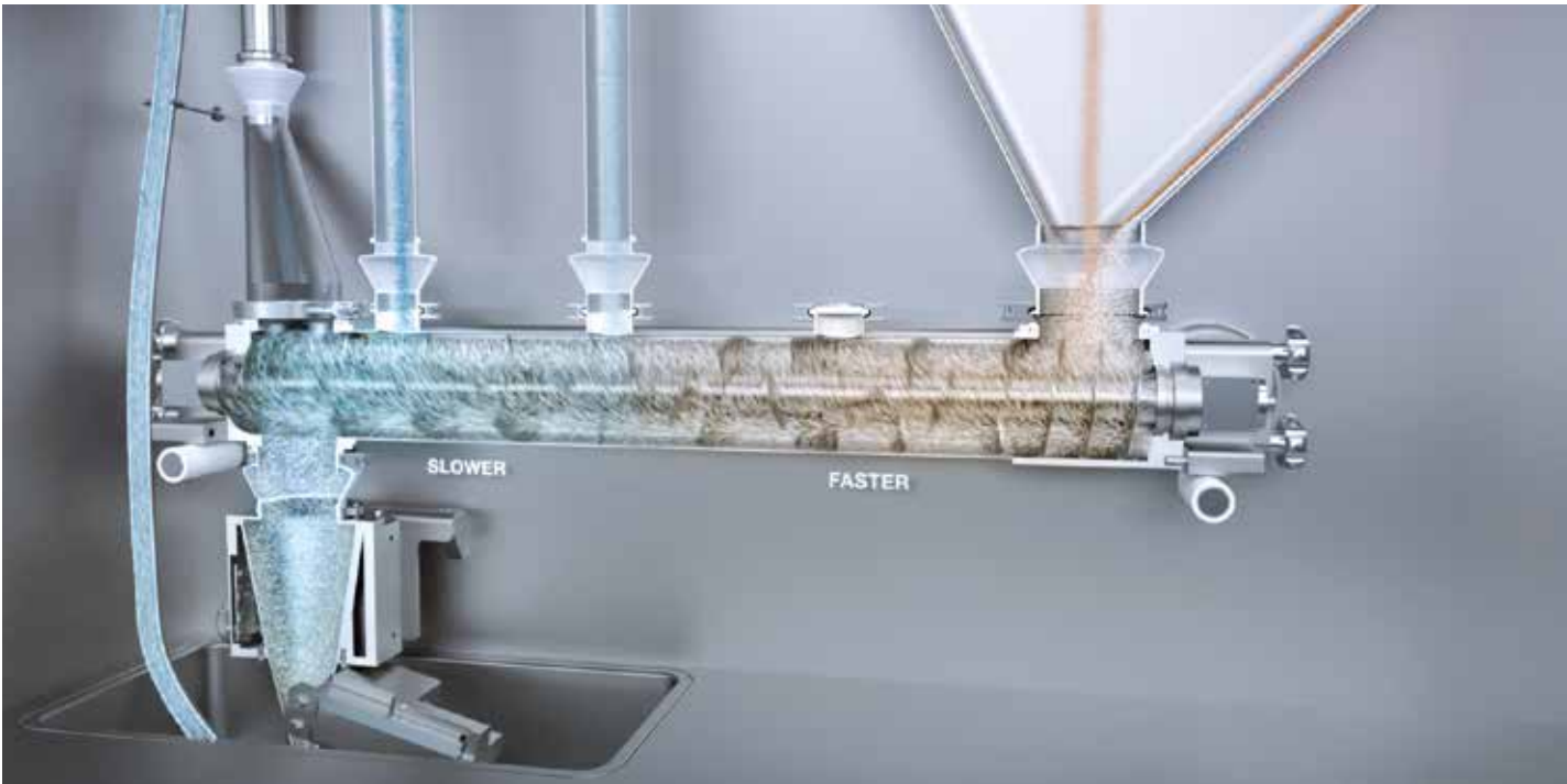
Two-zone blender (patent pending*): possibility to blend with high shear and low shear in defined zones
