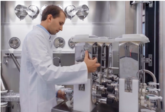
Tool-free: Components such as the blender, funnel, and feeder can be removed with just a few simple steps.
