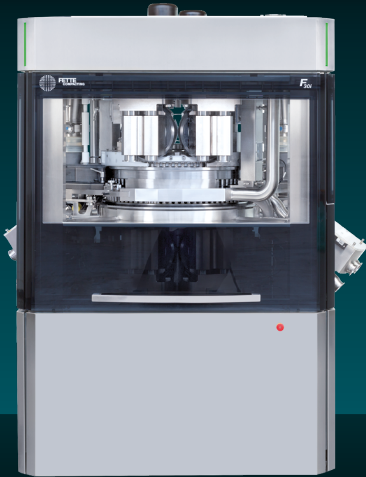
F30i The high-performance double rotary tablet press for maximum efficient production of large batches.
