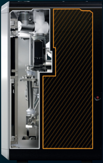
Strict separation of the process and technical area makes cleaning and product changeover of the dosing/blending unit much easier.
