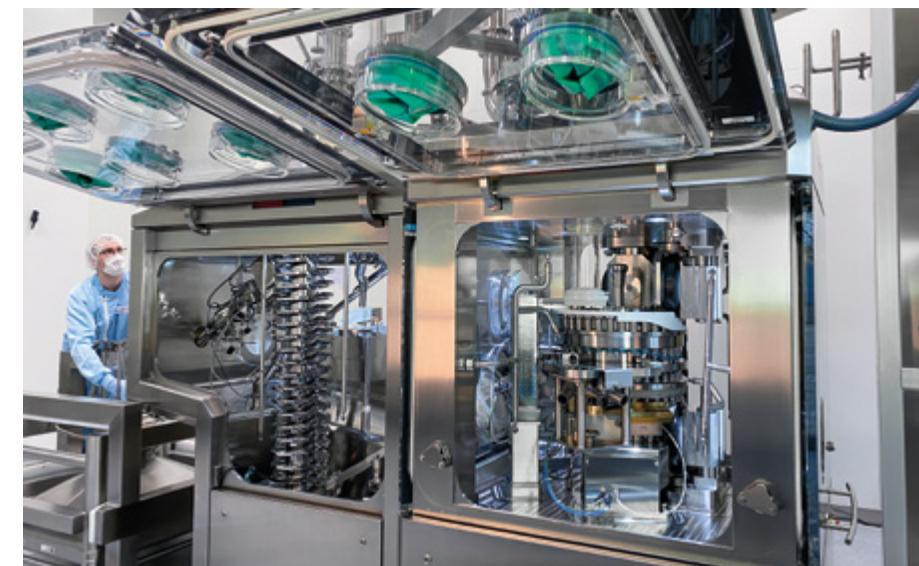
The second tablet press used by Boehringer Ingelheim in the factory is an FE55. The high-performance rotary press is suitable for a wide range of products and, with a maximum output of more than 600,000 tablets per hour, delivers particularly high performance. Its innovative filling system enables simple and safe feeding of complex product mixtures.
