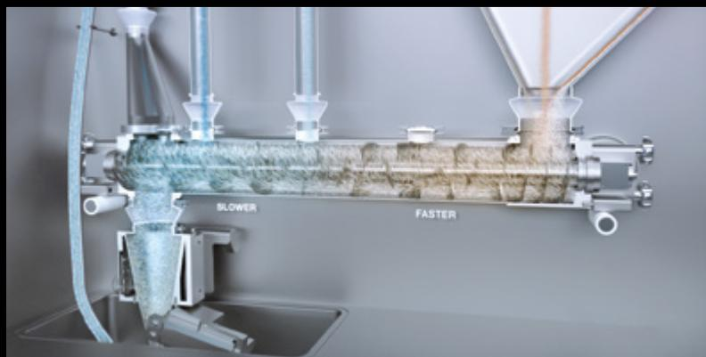
Possibility of mixing with high and low shear
