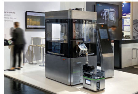
The CM-X allows tablet checking up to OEB Level 4. In September 2023, Fette Compacting presented the new Checkmaster for the first time at the Powtech in Nuremberg.
